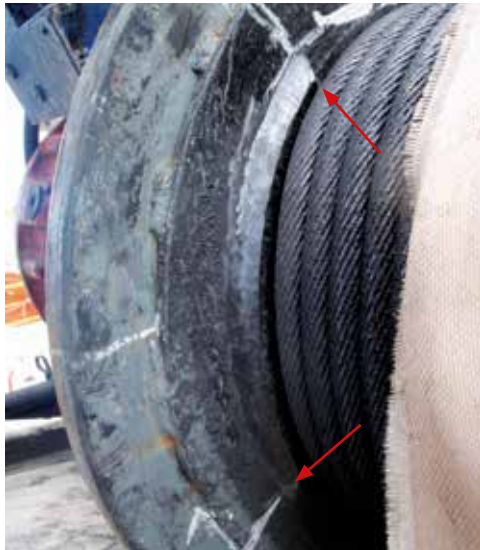
Figure 54 - Constriction that can cause rope distractions
