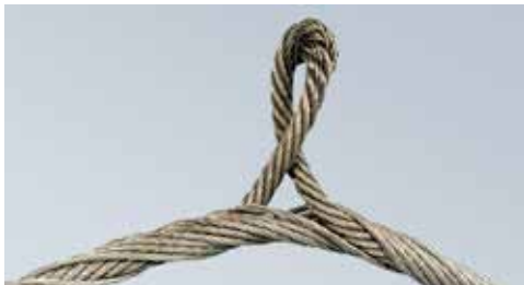
Figure 86 - Protrusion of inner rope
