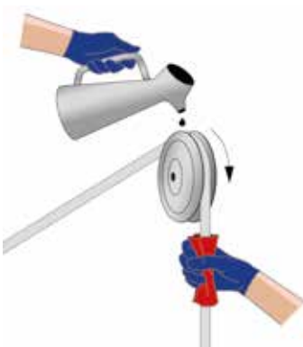
Figure 71 - manual lubrication located at sheave (symbolic illustration)
