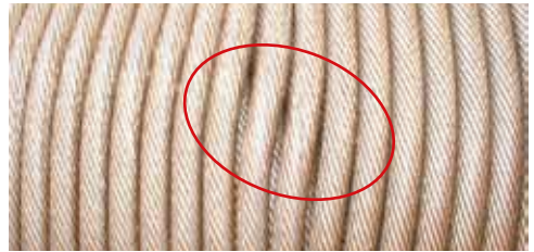
Figure 67 - loose spooling of rope in the outer layers
