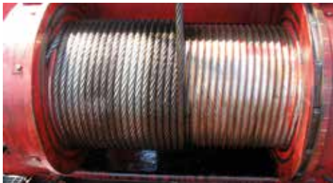
Figure 68 - drum ground should be visible for proper measurement
