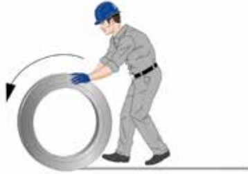
Figure 39 - proper unwinding off a coil
