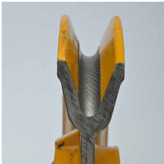
Figure 36 - negative impression of a used sheave
