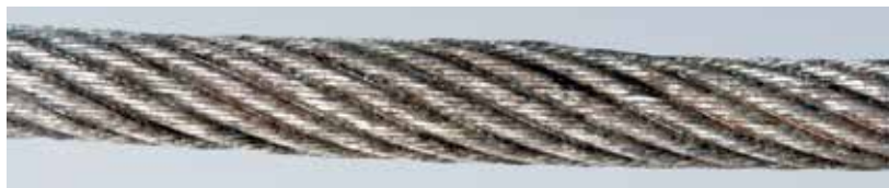
Figure 89 - Local increase in rope diameter due to core distortion
