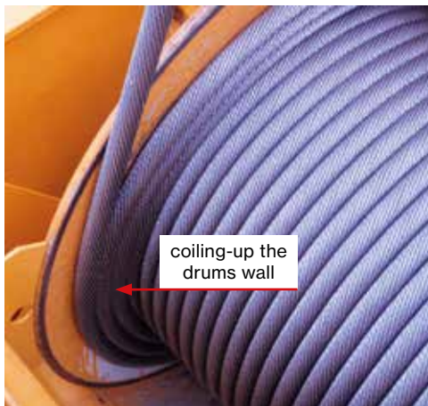
Figure 55 - coiling up the drums wall due to small fleet-angles
