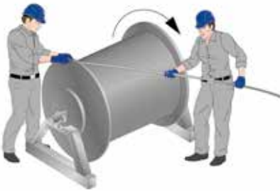
Figure 41 - correct unwinding off a bobbin
