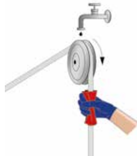
Figure 70 - automated lubrication located at sheave (symbolic illustration)
