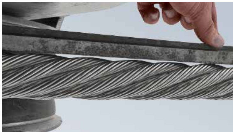
Figure 82 - How to measure waviness
