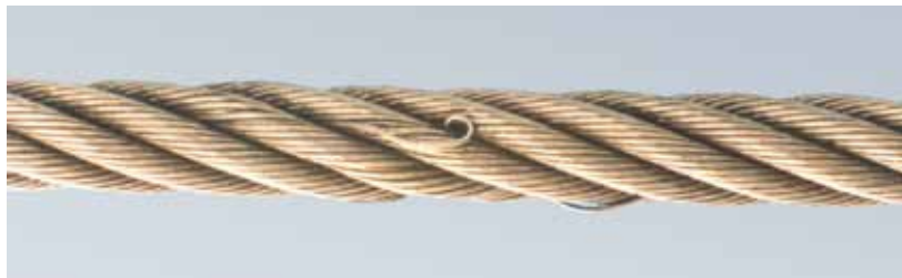
Figure 88 - Wire protrusion in loops
