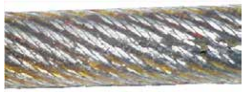
Figure 65 - Increased rope wear caused by too narrow spooling
