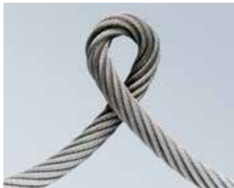
Figure 95 - Kink (tightened loop)
