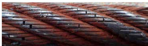
Figure 80 - Fretting corrosion due to inter-strand contact
