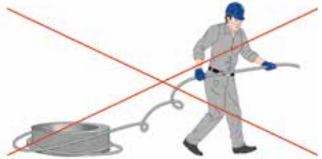
Figure 40 - improper unwinding off a coil
