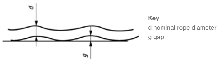
Figure 83 - parameters to evaluate waviness
