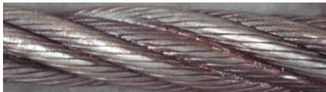
Figure 76 - Local reduction in rope diameter (sunken strand)
