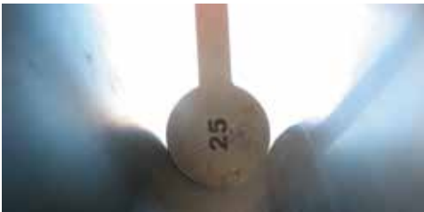
Figure 34 - act. groove diameter 25.0mm
