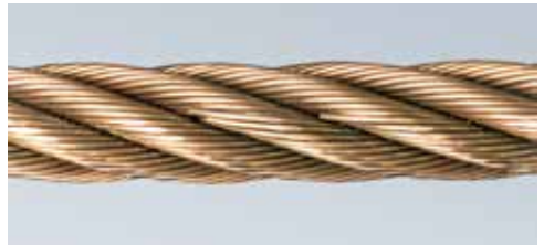
Figure 75 - Valley wire breaks
