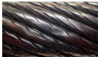
Figure 77 - Uniform diameter reduction may be caused by external wear
