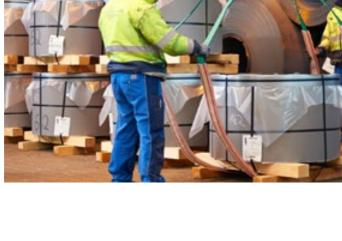
PowerStar – flat sling with "measurable" load capacity
